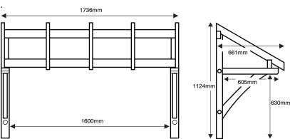
Cheshire Mouldings Porch Canopies have been structurally tested to hold a maximum weight loading of 50kg/m2 Structural calculations are based on fixing to masonry surfaces such as brick, block and stone.
