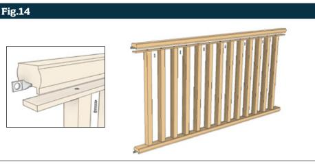
Place assembled rail/spindle infill between and to front of decking posts and rest on 40mm blocks so that the Deckit brackets are up against the post faces **(Fig.15)**. Mark 4 bracket hole centre positions on the newel posts and off set vertical centreline by 2mm.
