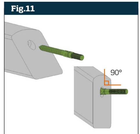
To fix over post connector to top of intermediate newel post, apply bead of multi purpose adhesive to top of newel. Offer over post connector P1 (1) onto top of newel post. Pilot drill through 2 x screw holes using 3.5mm dia bit. Secure connector to top of post using 2 off, 4.8mm x 40mm screws supplied (**Fig.12**). Temporarily fit over post connector P2 (2) to base using M6 bolt and nut supplied but do not overtighten (**Fig.13**).
