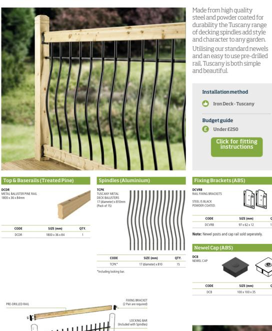
Made from high quality powder coated steel these spindles offer strength and style whilst providing a modern look and feel to decking.
