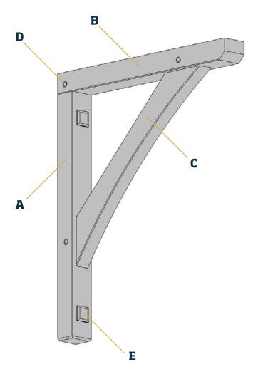
**Please note:** when gallows brackets CP300 are used with Cheshire Mouldings Apex Porch range, the canopies have been structurally tested to hold a maximum weight loading of **50kg/m²**.
