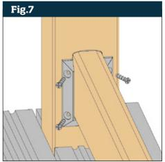
Offer rail hanger brackets to each end of the top rail. Pilot drill through back bracket holes and secure with screws supplied. Draw a horizontal line 30mm down from top of top rail to approx. 50mm long. This will be used to set height of top rail to spindle tops **(Fig.8)**.
