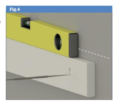
Take shelf and place next to wall batten ensuring that ends are flush. Using a square or straight edge, extend wall batten hole centre locations across to top of shelf. Drill a Ø4.5mm countersunk hole through, 9mm from back edge of shelf and another at 35mm from back of shelf (**Fig 5**).
