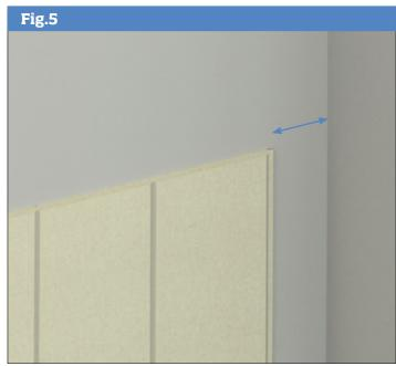
Remove second to last panel and offer cut piece into it. Apply adhesive to the back of the panels. Offer panels at an angle into position and press into place **(Fig 6)**.
