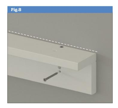
Offer each numbered bracket up to wall batten and shelf ensuring the bracket dowel locates in the 8mm hole. While supporting the bracket, insert screws down through previously drilled holes in shelf to secure **(Fig 9)**.
