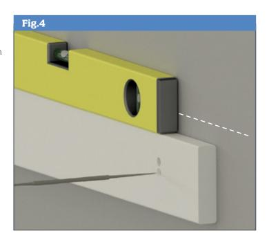
Take shelf and place next to wall batten ensuring that ends are flush. Using a square or straight edge, extend wall batten hole centre locations across to top of shelf. Drill a Ø4.5mm countersunk hole through, 9mm from back edge of shelf and another at 35mm from back of shelf (**Fig 5**).
