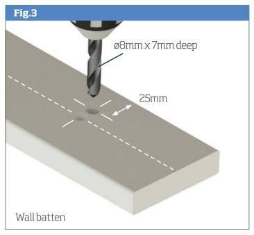
Take wall batten, ensuring ø8mm holes are to the top and offer up to preferred height on wall, allowing 18mm for the top shelf. Check horizontal using a spirit level then mark through each of the previously drilled ø4.5mm holes using a scriber or screw to establish location for wall fixings. Remove wall batten and drill and plug marked points using appropriate plugs to suit wall construction (Fig 4).
